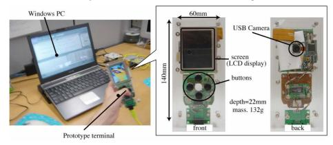
Fig. 8. Prototype system
